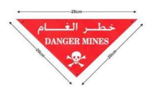
The unmarked side of the sign shall face the inside of the hazardous area and the marked side shall be visible from the outside of the area. The sign should be securely fastened to a fence or a post at intervals not greater than 30m.
